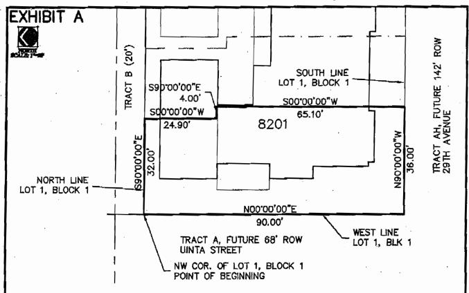
BEGINNING AT THE NORTHWEST CORNER OF SAID LOT 1, BLOCK 1, STAPLETON FILING NO. 5; THENCE S 90'00'00" E, A DISTANCE OF 32.00 FEET; THENCE S 00'00'00" W, A DISTANCE OF 24.90 FEET; THENCE S 90'00'00" E, A DISTANCE OF 4.00 FEET; THENCE S 00'00'00" W, A DISTANCE OF 65.10 FEET; THENCE N 90'00'00" W, A DISTANCE OF 36.00 FEET; THENCE N 00'00'00" E, A DISTANCE OF 90.00 FEET TO THE POINT OF BEGINNING.
