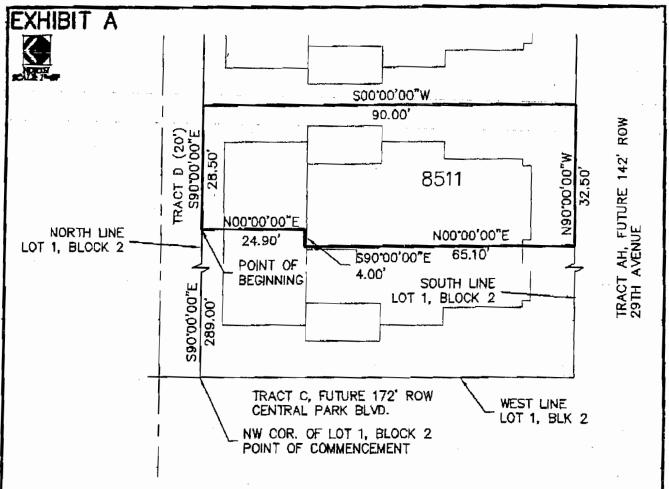
COMMENCING AT THE NORTHWEST CORNER OF SAID LOT 1, BLOCK 2, STAPLETON FILING NO. 5; THENCE S 90'00'00" E, A DISTANCE OF 289.00 FEET TO THE POINT OF BEGINNING; THENCE S 90'00'00" W, A DISTANCE OF 90.00 FEET; THENCE N 90'00'00" W, A DISTANCE OF 32.50 FEET; THENCE N 90'00'00" E, A DISTANCE OF 65.10 FEET; THENCE N 00'00'00" E, A DISTANCE OF 65.10 FEET; THENCE S 90'00'00" E, A DISTANCE OF 4.00 FEET; THENCE N 00'00'00" E, A DISTANCE OF 24.90 FEET TO THE POINT OF BEGINNING.
