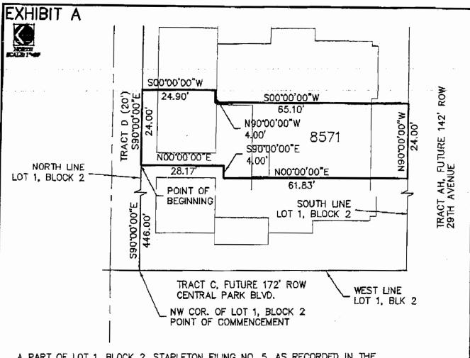
ICING AT THE NORTHWEST CORNER OF SAID LOT 1, BLOCK 2, STAPLETON FILING NO. 5; S 90'00'00" E, A DISTANCE OF 446.00 FEET TO THE POINT OF BEGINNING; S 90'00'00" E, A DISTANCE OF 24.00 FEET; S 00'00'00" W, A DISTANCE OF 4.00 FEET; N 90'00'00" W, A DISTANCE OF 65.10 FEET; N 90'00'00" W, A DISTANCE OF 65.10 FEET; N 90'00'00" E, A DISTANCE OF 61.83 FEET; N 90'00'00" E, A DISTANCE OF 61.83 FEET; S 90'00'00" E, A DISTANCE OF 4.00 FEET; N 00'00'00" E, A DISTANCE OF 28.17 FEET TO THE POINT OF BEGINNING OF
