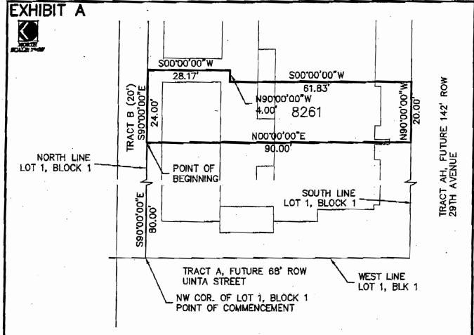
COMMENCING AT THE NORTHWEST CORNER OF SAID LOT 1, BLOCK 1, STAPLETON FILING NO. 5; THENCE S 90°00'00" E, A DISTANCE OF 80.00 FEET TO THE POINT OF BEGINNING; THENCE S 90°00'00" W, A DISTANCE OF 28.17 FEET; THENCE N 90°00'00" W, A DISTANCE OF 4.00 FEET; THENCE N 90°00'00" W, A DISTANCE OF 61.83 FEET; THENCE N 90°00'00" W, A DISTANCE OF 61.83 FEET; THENCE N 90°00'00" W, A DISTANCE OF 20.00 FEET; THENCE N 00°00'00" E, A DISTANCE OF 90.00 FEET TO THE POINT OF BEGINNING.
