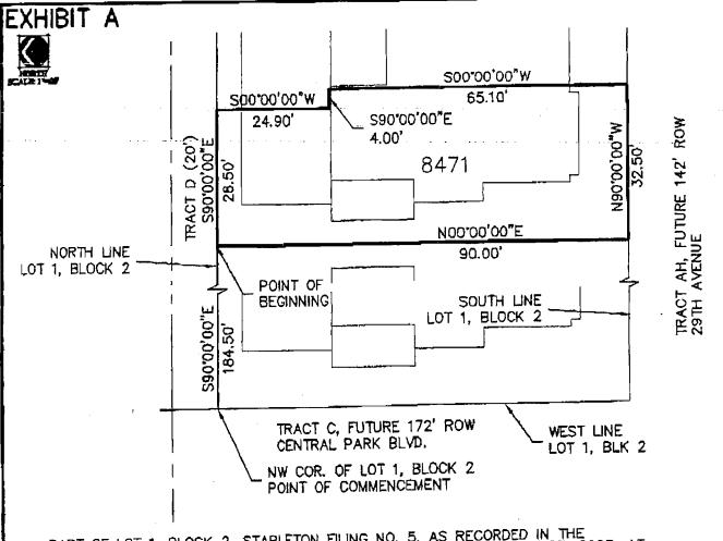
COMMENCING AT THE NORTHWEST CORNER OF SAID LOT 1, BLOCK 2, STAPLETON FILING NO. 5; THENCE S 90'00'00" E, A DISTANCE OF 184.50 FEET TO THE POINT OF BEGINNING; THENCE S 90'00'00" W, A DISTANCE OF 24.90 FEET; THENCE S 90'00'00" E, A DISTANCE OF 4.00 FEET; THENCE S 90'00'00" W, A DISTANCE OF 4.00 FEET; THENCE S 00'00'00" W, A DISTANCE OF 65.10 FEET; THENCE N 90'00'00" W, A DISTANCE OF 32.50 FEET; THENCE N 90'00'00" W, A DISTANCE OF 90.00 FEET TO THE POINT OF BEGINNING.
