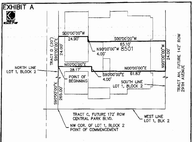
NG AT THE NORTHWEST CORNER OF SAID LOT 1, BLOCK 2, STAPLETON FILING NO. 5; 90°00'00" E, A DISTANCE OF 265.00 FEET TO THE POINT OF BEGINNING; 90°00'00" W, A DISTANCE OF 24.90 FEET; 90°00'00" W, A DISTANCE OF 4.00 FEET; 00°00'00" W, A DISTANCE OF 65.10 FEET; 90°00'00" W, A DISTANCE OF 65.10 FEET; 90°00'00" W, A DISTANCE OF 65.10 FEET; 90°00'00" F, A DISTANCE OF 61.83 FEET;
