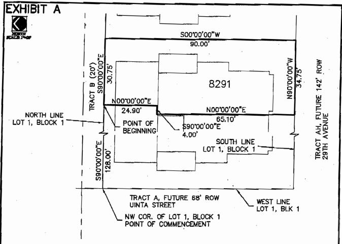
COMMENCING AT THE NORTHWEST CORNER OF SAID LOT 1, BLOCK 1, STAPLETON FILING NO. 5; THENCE S 90°00'00" E, A DISTANCE OF 128.00 FEET TO THE POINT OF BEGINNING; THENCE S 90°00'00" W, A DISTANCE OF 90.00 FEET; THENCE N 90°00'00" W, A DISTANCE OF 34.75 FEET; THENCE N 90°00'00" E, A DISTANCE OF 65.10 FEET; THENCE N 00°00'00" E, A DISTANCE OF 4.00 FEET; THENCE S 90°00'00" E, A DISTANCE OF 4.00 FEET; THENCE N 00°00'00" E, A DISTANCE OF 24.90 FEET TO THE POINT OF BEGINNING.
