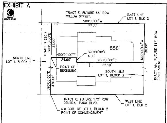
COMMENCING AT THE NORTHWEST CORNER OF SAID LOT 1, BLOCK 2, STAPLETON FILING NO. 5; THENCE S 90'00'00" E, A DISTANCE OF 470.00 FEET; THENCE S 90'00'00" W, A DISTANCE OF 90.00 FEET; THENCE N 90'00'00" W, A DISTANCE OF 36.00 FEET; THENCE N 90'00'00" W, A DISTANCE OF 36.00 FEET; THENCE N 00'00'00" E, A DISTANCE OF 65.10 FEET; THENCE N 90'00'00" E, A DISTANCE OF 4.00 FEET; THENCE N 90'00'00" E, A DISTANCE OF 24.90 FEET TO THE POINT OF BEGINNING.
