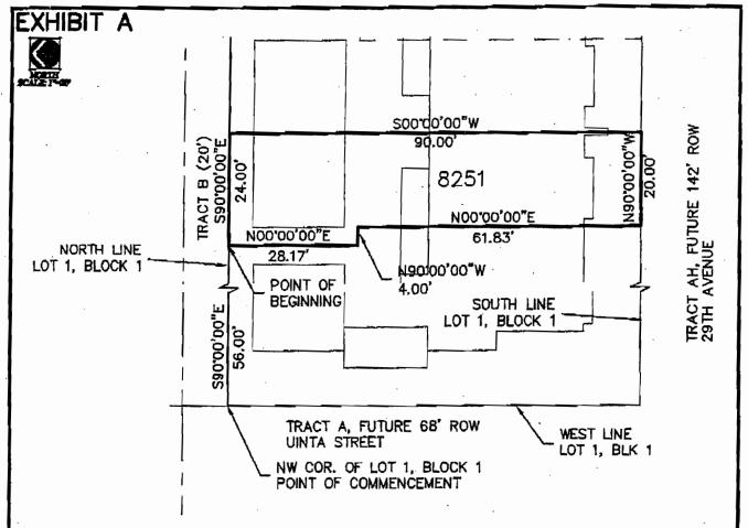
COMMENCING AT THE NORTHWEST CORNER OF SAID LOT 1, BLOCK 1, STAPLETON FILING NO. 5; THENCE S 90'00'00" E, A DISTANCE OF 56.00 FEET TO THE POINT OF BEGINNING; THENCE S 90'00'00" E, A DISTANCE OF 24.00 FEET; THENCE S 00'00'00" W, A DISTANCE OF 90.00 FEET; THENCE N 90'00'00" W, A DISTANCE OF 20.00 FEET; THENCE N 00'00'00" E, A DISTANCE OF 61.83 FEET; THENCE N 90'00'00" W, A DISTANCE OF 4.00 FEET; THENCE N 00'00'00" E, A DISTANCE OF 28.17 FEET TO THE POINT OF BEGINNING.
