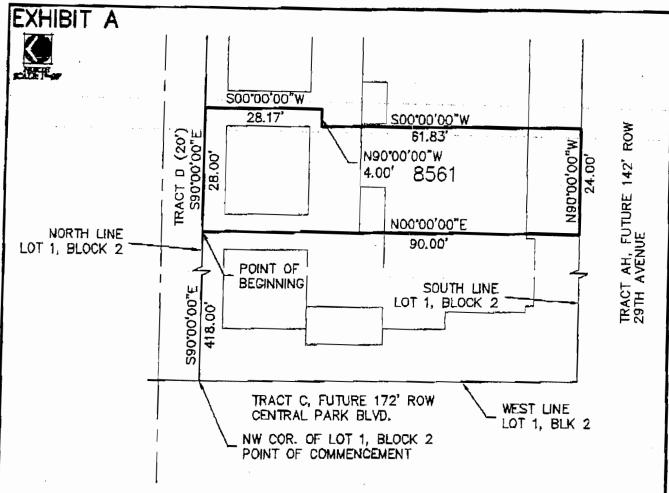
COMMENCING AT THE NORTHWEST CORNER OF SAID LOT 1, BLOCK 2, STAPLETON FILING NO. 5; THENCE S 90°00'00" E, A DISTANCE OF 418.00 FEET TO THE POINT OF BEGINNING; THENCE S 90°00'00" E, A DISTANCE OF 28.00 FEET; THENCE S 00°00'00" W, A DISTANCE OF 28.17 FEET; THENCE N 90°00'00" W, A DISTANCE OF 4.00 FEET; THENCE N 90°00'00" W, A DISTANCE OF 61.83 FEET; THENCE N 90°00'00" W, A DISTANCE OF 24.00 FEET; THENCE N 00°00'00" E, A DISTANCE OF 90.00 FEET TO THE POINT OF BEGINNING.
