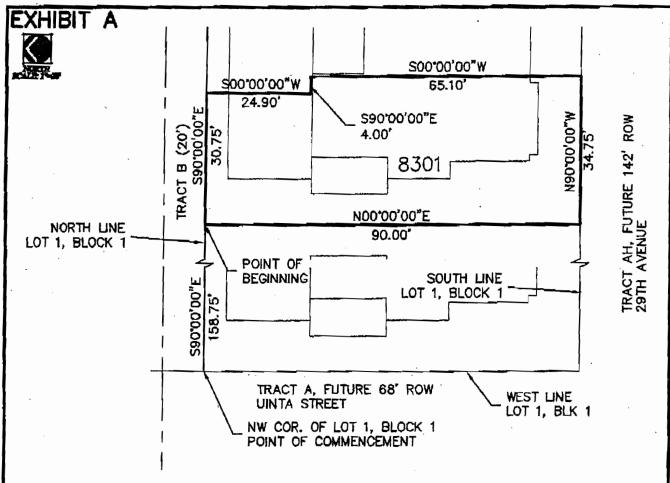
COMMENCING AT THE NORTHWEST CORNER OF SAID LOT 1, BLOCK 1, STAPLETON FILING NO. 5; THENCE S 90'00'00" E, A DISTANCE OF 158.75 FEET TO THE POINT OF BEGINNING; THENCE S 90'00'00" W, A DISTANCE OF 24.90 FEET; THENCE S 90'00'00" E, A DISTANCE OF 4.00 FEET; THENCE S 90'00'00" W, A DISTANCE OF 65.10 FEET; THENCE N 90'00'00" W, A DISTANCE OF 34.75 FEET; THENCE N 90'00'00" E, A DISTANCE OF 90.00 FEET TO THE POINT OF BEGINNING.
